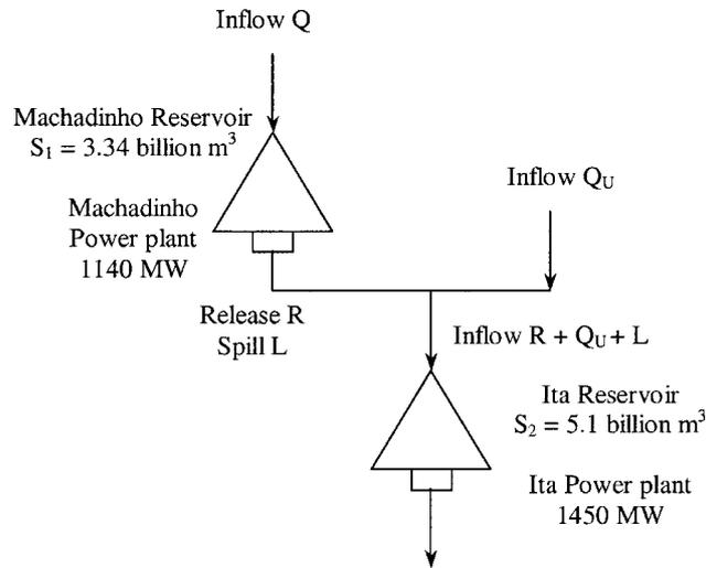
Figure 3. Schematic Representation of the Machadinho-Ita System (MIS).
