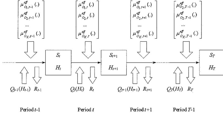
Figure 1. Reservoir Operation in a Stochastic and Fuzzy Environment.
