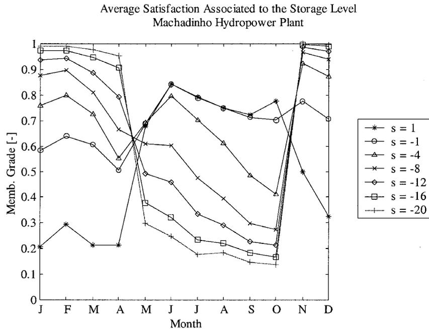
Figure 8. Simulated Average Satisfaction Associated to the Storage Level.
